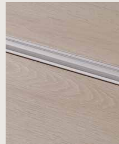
MULTIFUNCTIONAL PROFILE SILVER 1860 × 47 × 16 mm The Pergo multifunctional profile can level height differences for a smooth transition on to any other type of floor. Suitable for height differences of 0 – 12,3 mm. Surface: aluminium.
